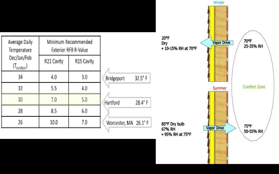
Tinterface = Tindoor – [(Tindoor – Toutdoor) x (Rcavity/Rtotal)]
