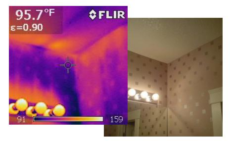
Missing insulation? Bulbs heating wall, ceiling? Top plate air leakage?
