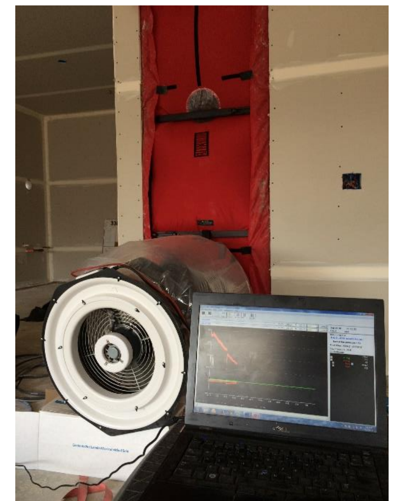
Blower door setup for pressurization
